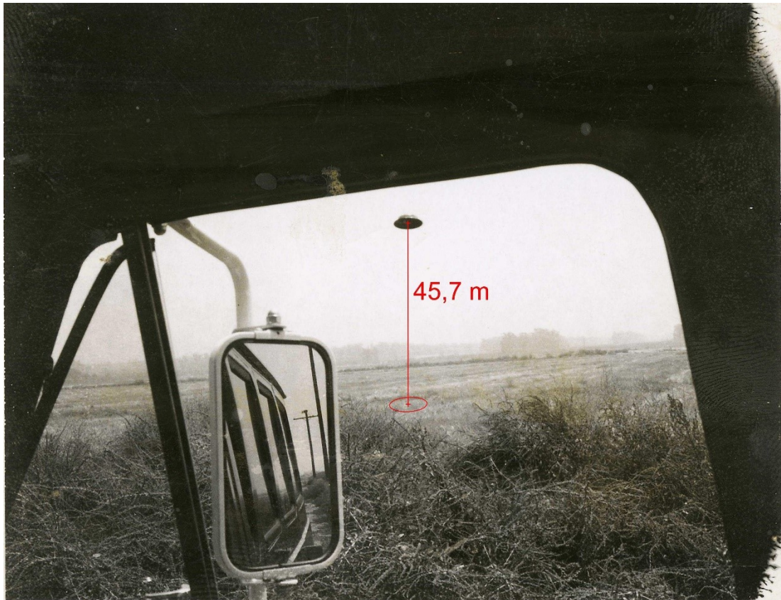
Photo H 2 : angle 2a = 9.37^\circ , distance D = 1.4 \times 201 = 281 m, height H = 45.7 m
