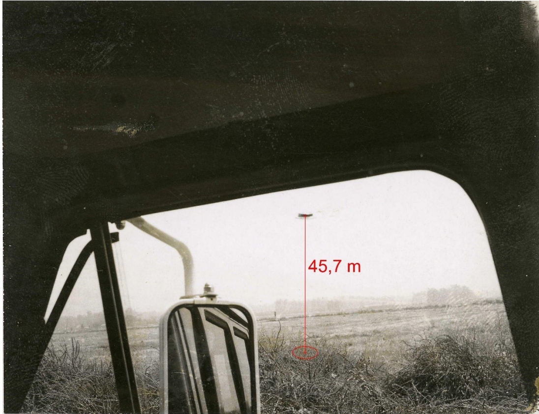
Photo H 3 : angle 2a = 10.10^\circ , distance D = 1.3 \times 201 = \mathbf{261 \text{ m}} , height H = \mathbf{45.7 \text{ m}}
