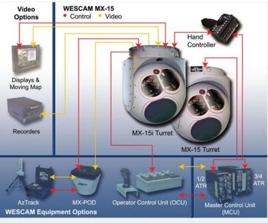
The Wescam MX-15 thermal imaging system. The same system used to capture the video. (Credit: Wescam)
